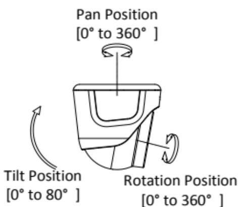
Figure 2-6 3-Axis Adjustment
