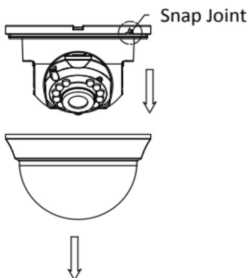
Figure 2. 9 Remove the Bubble
