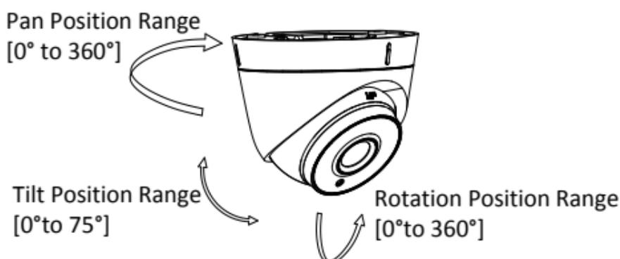
Figure 2. 8 3-axis Adjustment
