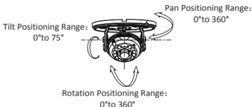
Figure 2. 12 3-axis Adjustment
