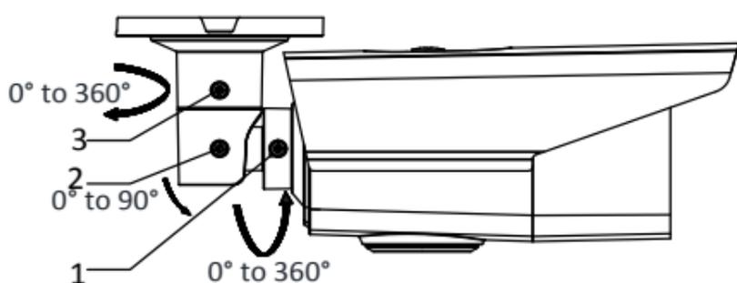
Figure 2. 3 3-Axis Adjustment
