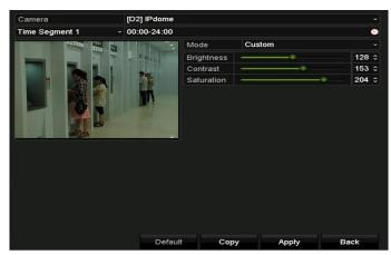
Figure 14-5 Image Settings Interface (IP Camera)
