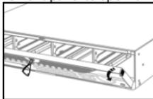
**Step 3** Insert the HDD until it is fixed firmly.
