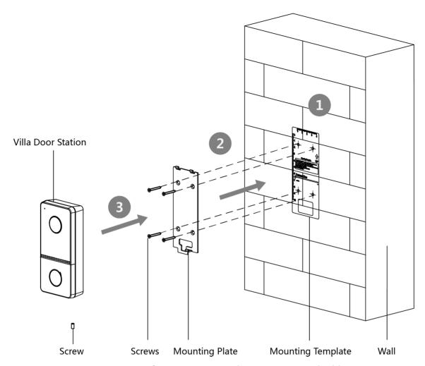
**Figure 3-4 Surface Mounting without Protective Shield**
