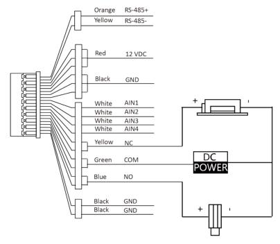
Figure 2-2 Door Lock Wiring
