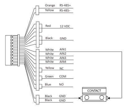
**Figure 2-3 Door Contact Wiring**
