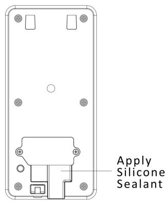
Figure 3-3 Apply Silicone Sealant
