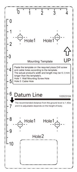
**Figure 3-2 Mounting Template**
