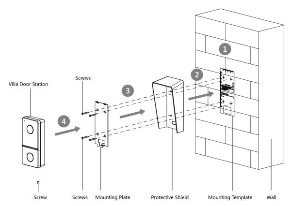
**Figure 3-6 Surface Mounting with Protective Shield**
