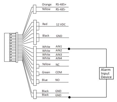
Figure 2-5 Alarm Input Device Wiring
