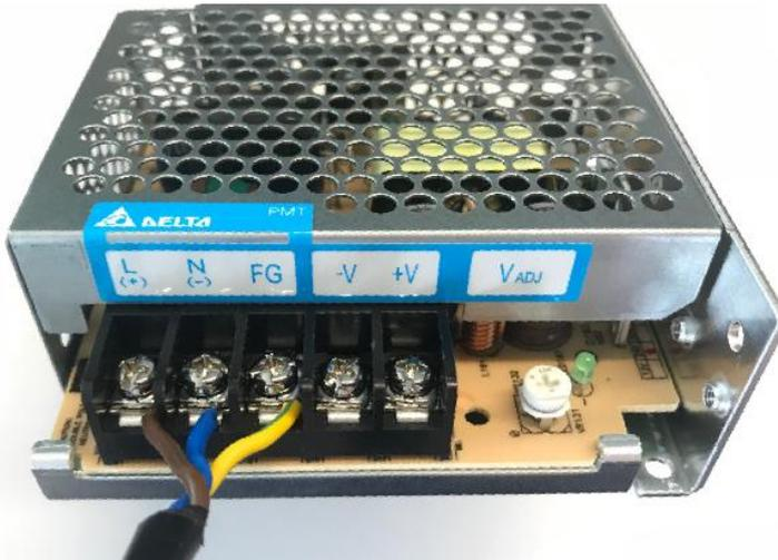
Figure 7-4 Connect to the Power Box
