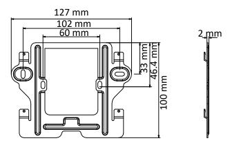
Figure 4-1 Wall Mounting Plate
