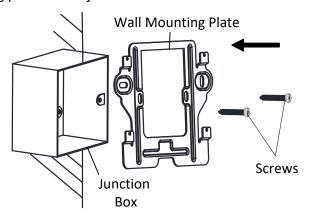
Figure 4-2 Installing the Plate
