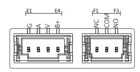
Figure 3-1 Terminals of Indoor Station
