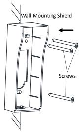
Figure 4-5 Installing the Shield
