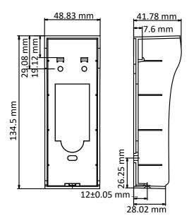
Figure 4-4 Wall Mounting Shield
