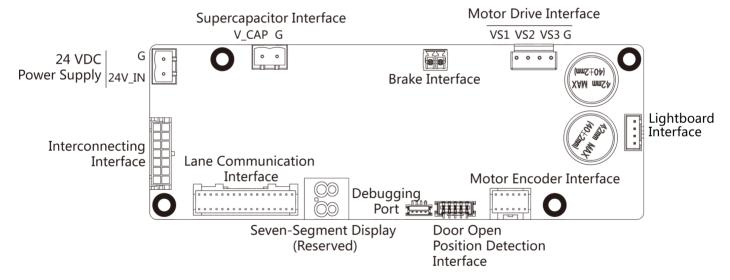
Figure 5-8 Sub Control Board
