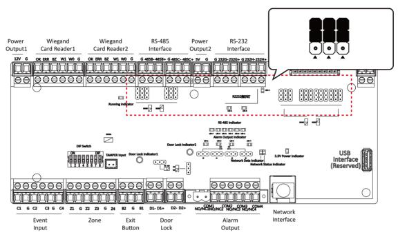
Figure 6-3 Jumper Cap Status of RS-232 Interface
