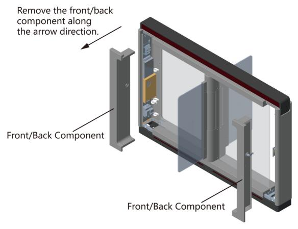
**Figure 4-3 Remove Components**
