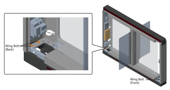
Figure 3-4 Loosen Wing Bolt
