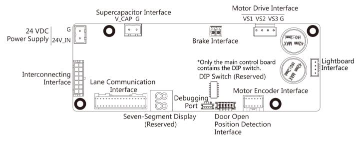
**Figure 5-7 Main Control Board**
