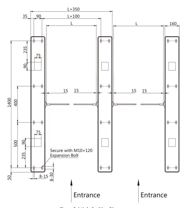
Figure 2-1 Hole Position Diagram
