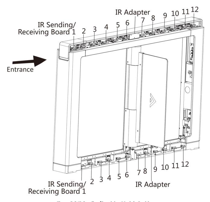
Figure 5-2 IR Sending/Receiving Module Position
