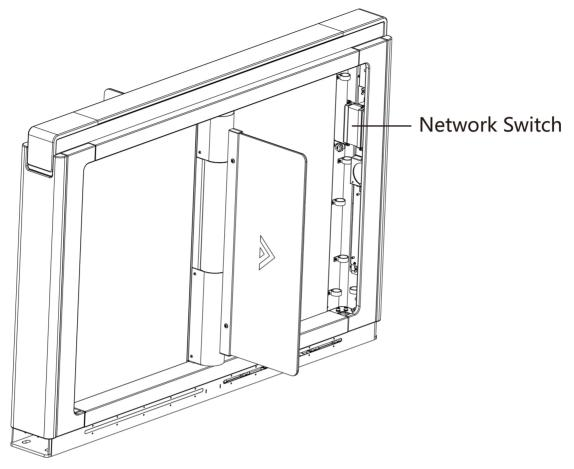
**Figure 5-5 Network Switch Position**
