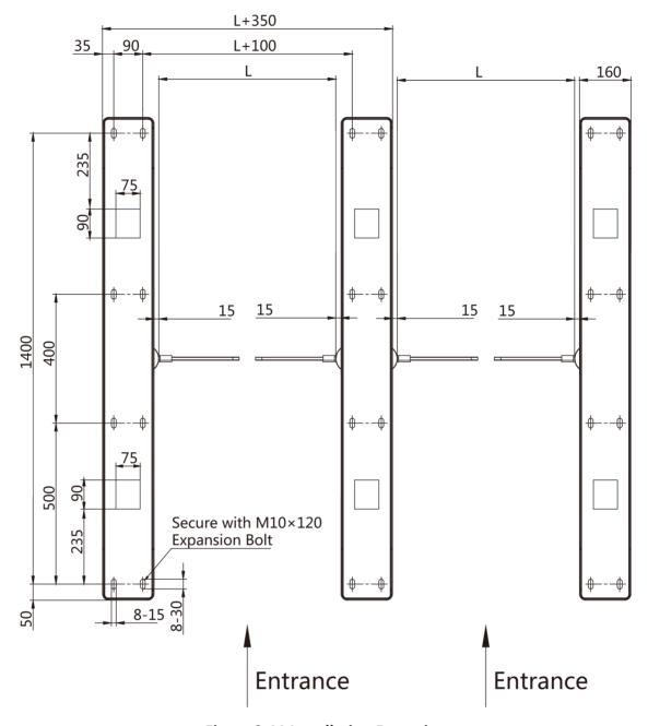
Figure 3-11 Installation Footprint
