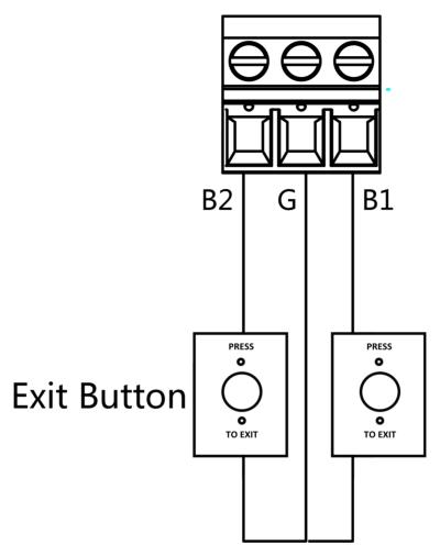
Figure 5-12 Exit Button Wiring
