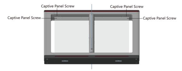
Figure 4-10 Loosen Captive Panel Screw
