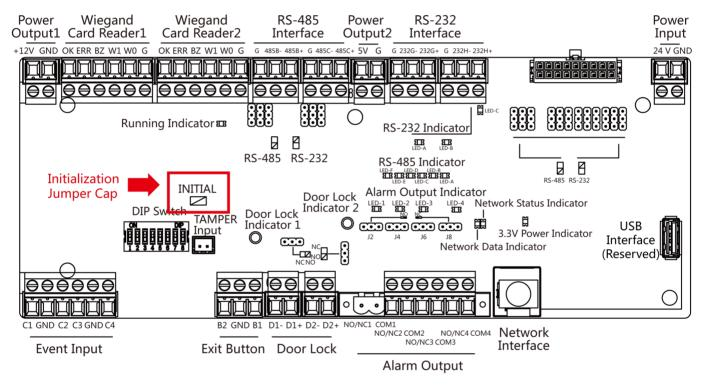
Figure 6-1 Initialization Jumper Cap
