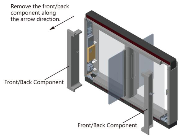
**Figure 3-3 Remove Components**
