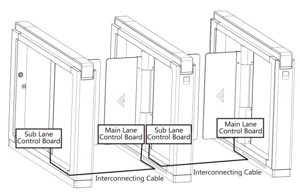
**Figure 5-4 Connect Interconnecting Cable**
