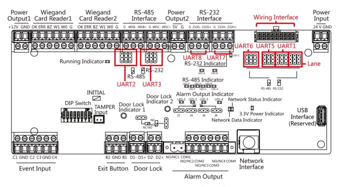
Figure 5-10 Access Control Board
