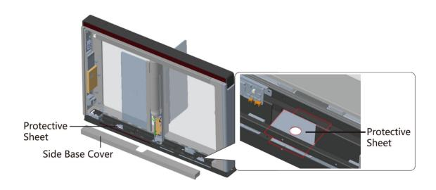
**Figure 3-9 Disassemble Two Protective Sheets**
