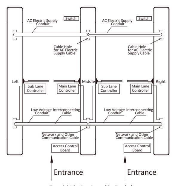
**Figure 2-3 Wire Face Recognition Terminal**
