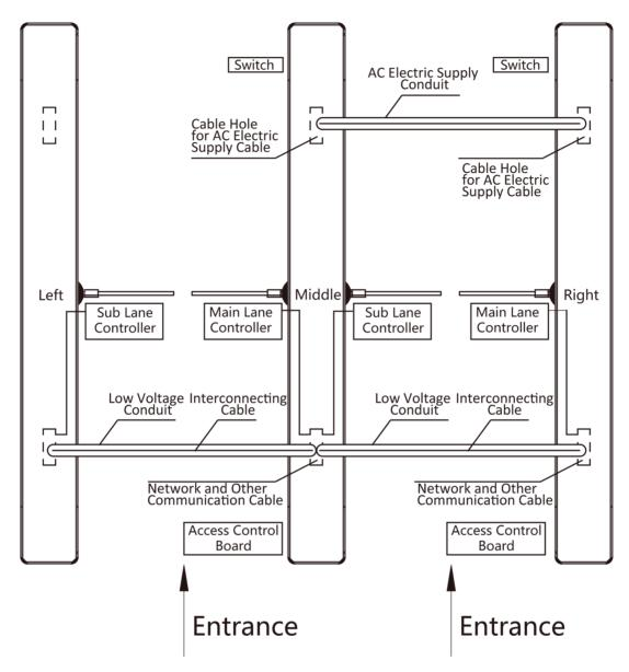
Figure 2-2 System Wiring Diagram (General Wiring)
