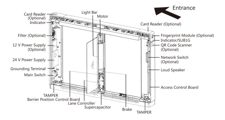
Figure 5-1 Components Diagram
