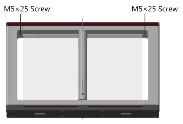
Figure 4-7 M5×25 Screws Position
