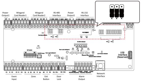
Figure 6-2 Jumper Cap Status of RS-485 Interface
