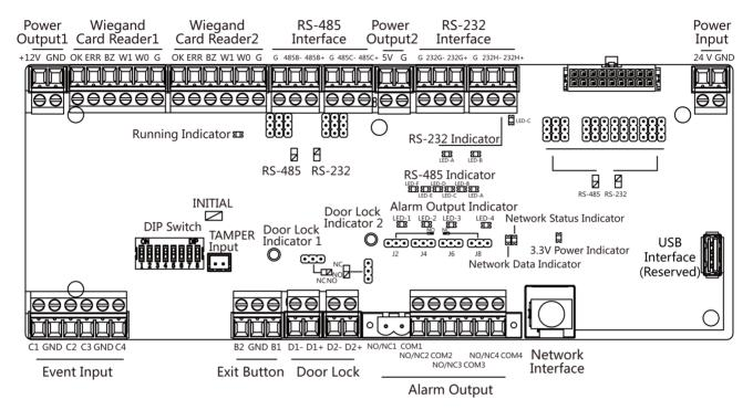
**Figure 5-9 Access Control Board**
