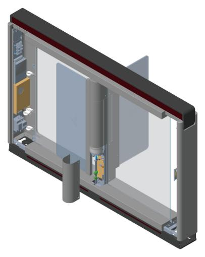
**Figure 3-7 Remove Motor Bottom Cover**
