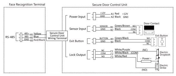
Figure 4-3 Secure Door Control Unit Wiring
