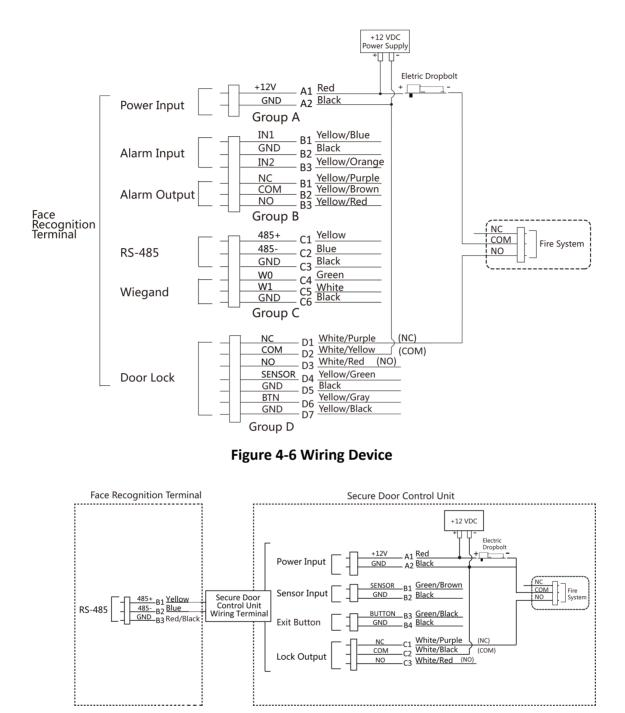
Figure 4-7 Wiring Secure Door Control Unit
