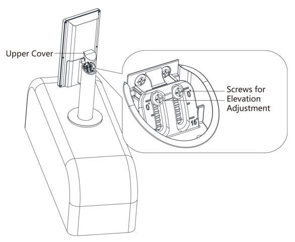
Figure 3-4 Adjust Elevation
