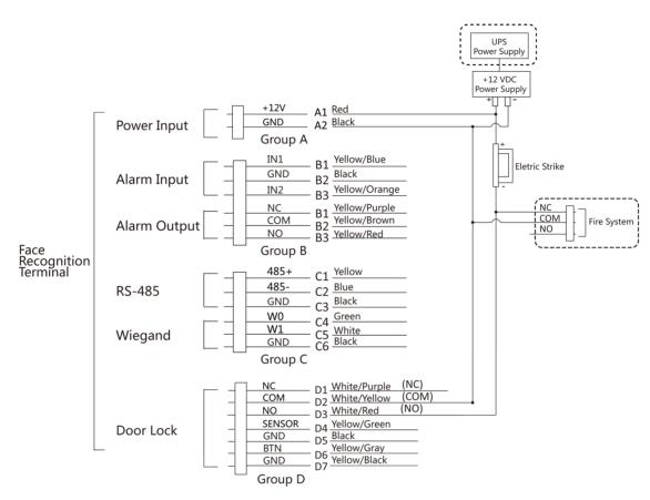
Figure 4-8 Device Wiring
