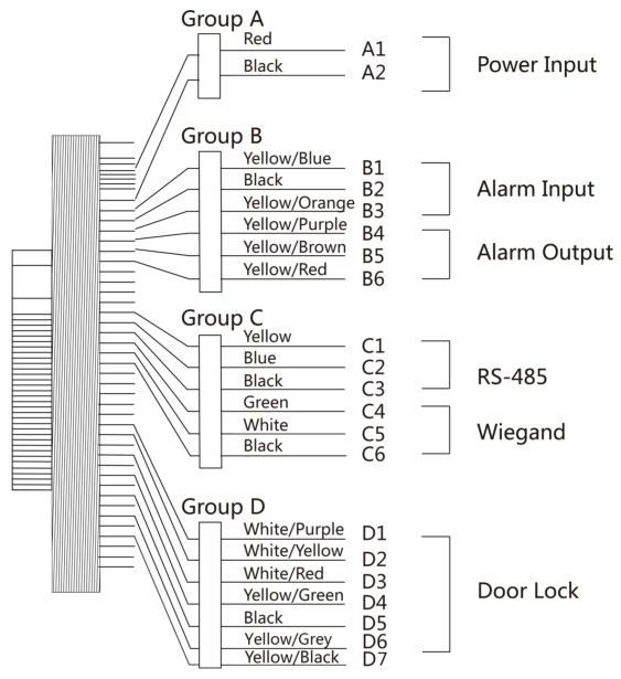
Figure 4-1 Terminal Diagram
