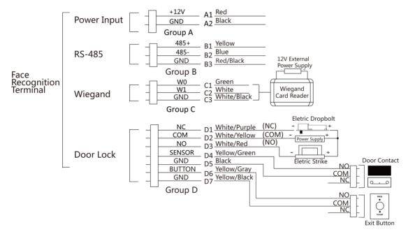
Figure 4-1 Device Wiring
