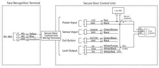
Figure 4-6 Wiring Secure Door Control Unit
