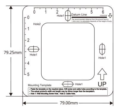
Figure 3-1 Mounting Template
