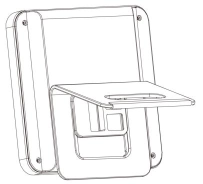
Figure 3-5 Align Bracket and Device
