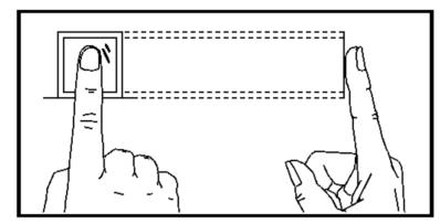
You should press your finger on the scanner horizontally. The center of your scanned finger should align with the scanner center.
