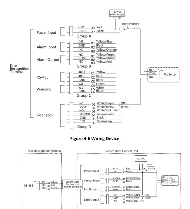
Figure 4-7 Wiring Secure Door Control Unit
