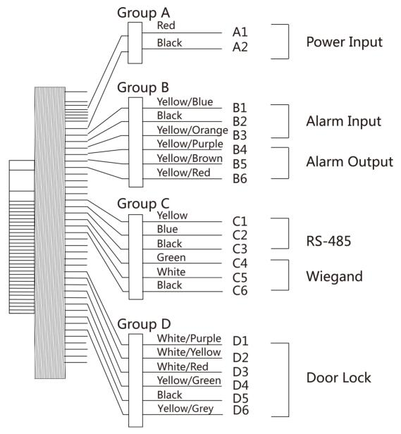
Figure 4-1 Terminal Diagram
