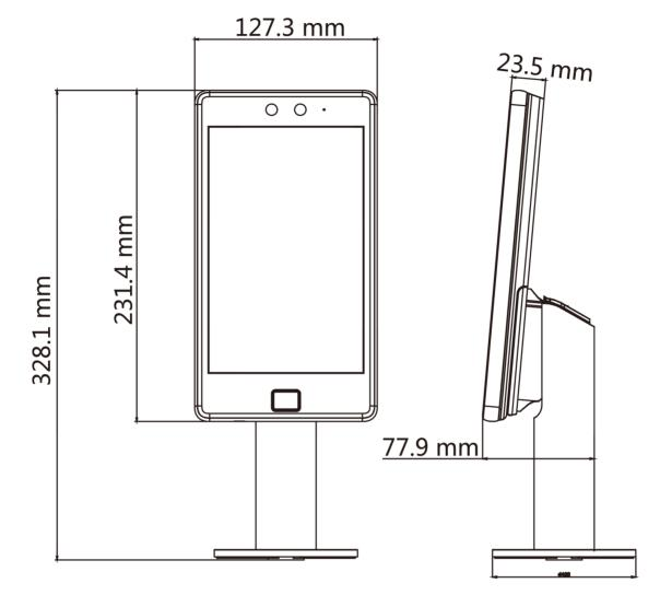
Figure D-2 Dimension with Bracket
