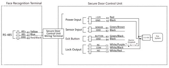
Figure 4-5 Wire Secure Door Control Unit
