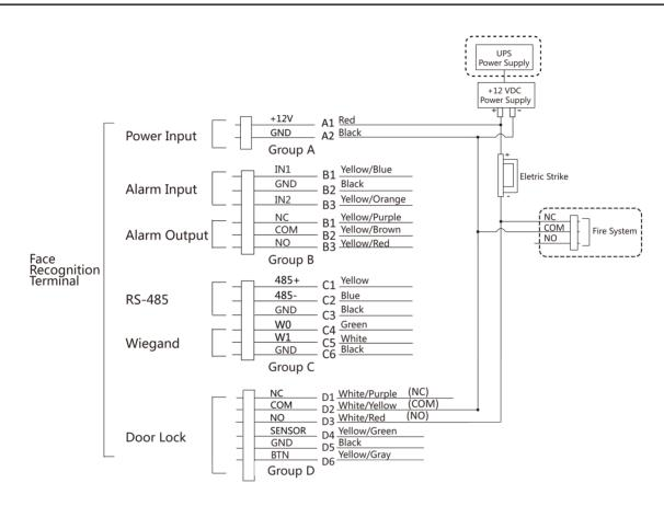
Figure 4-8 Device Wiring
