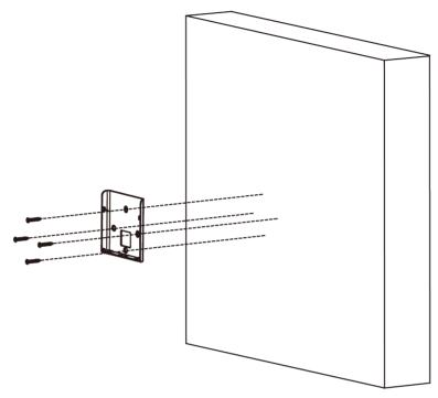
Figure 3-2 Install Mounting Plate
