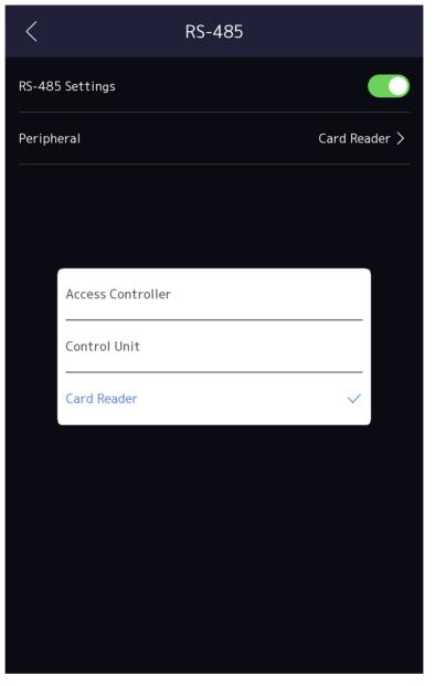
Figure 7-7 Set RS-485 Parameters
