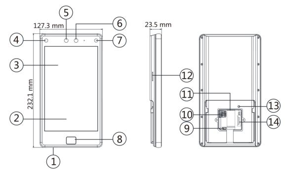
Figure 2-1 Face Recognition Terminal Diagram
