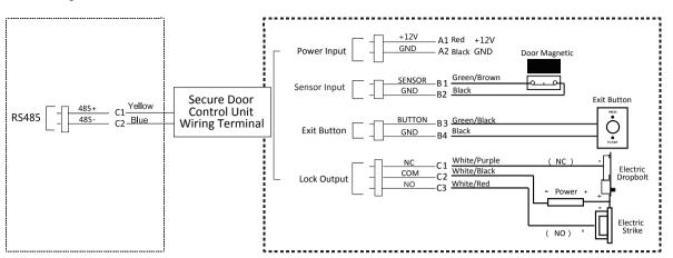
Note: The secure door control unit should connect to an external power supply separately.
