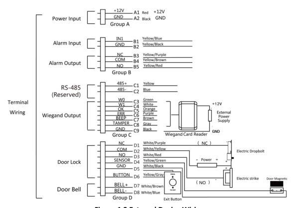
Figure 4-2 External Device Wiring
