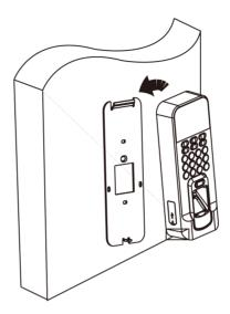
Figure 5-3 Install Device
