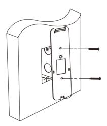
Figure 5-2 Install Mounting Plate
