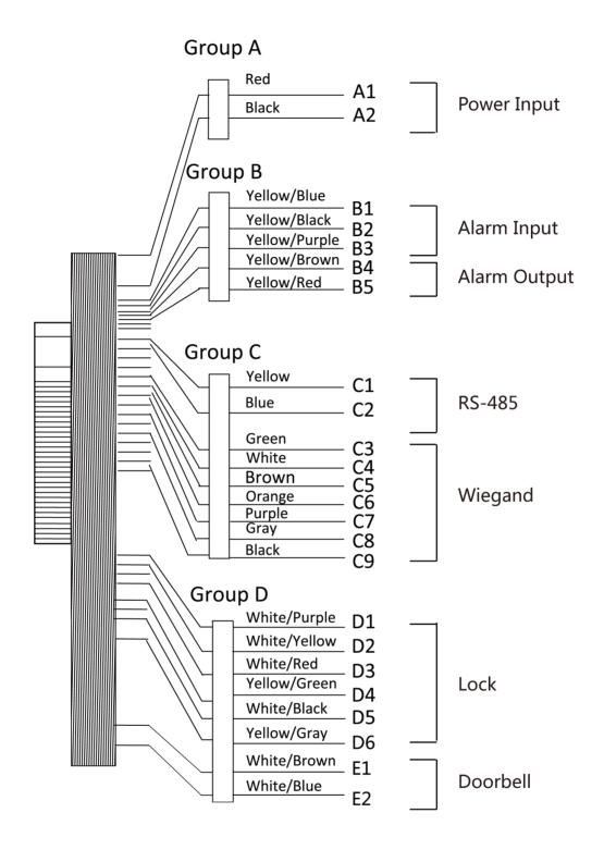
Figure 4-1 Terminal Diagram
