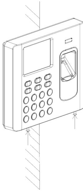
**Figure 3-6 Secure Device**
