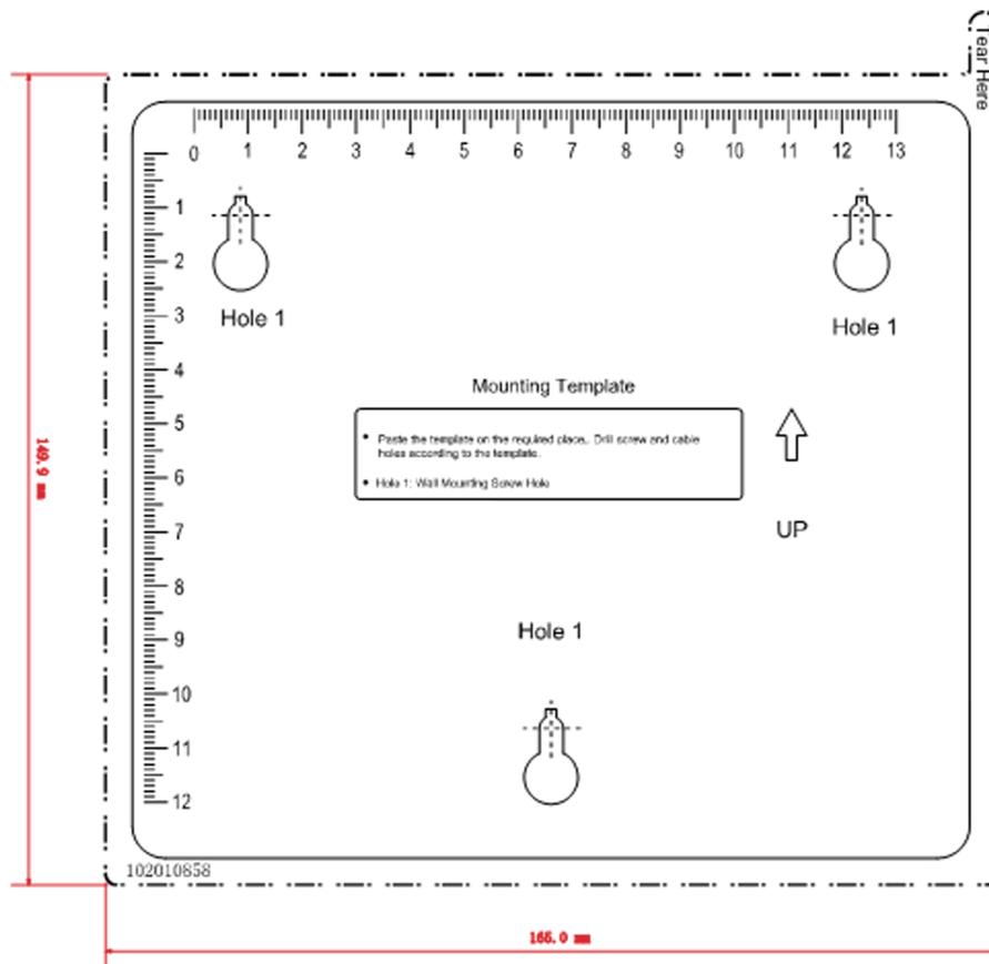
Figure 3-1 Mounting Template
