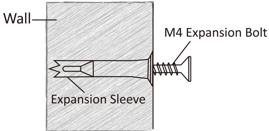
**Figure 3-2 Install Screws**
