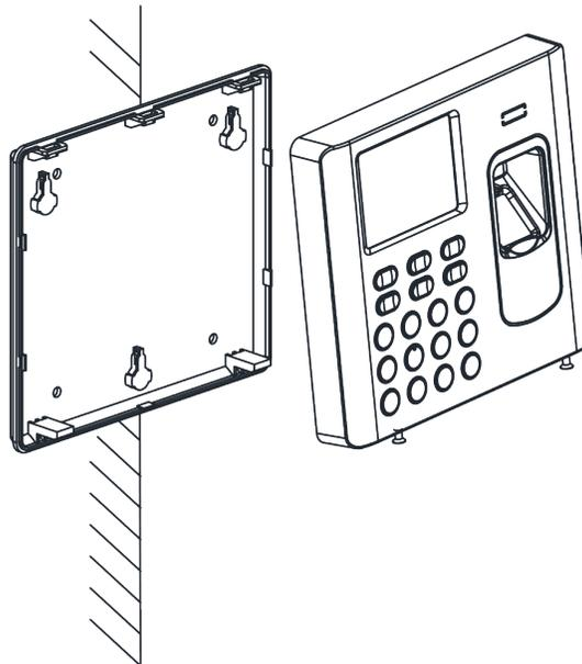
**Figure 3-5 Install Front Cover**
