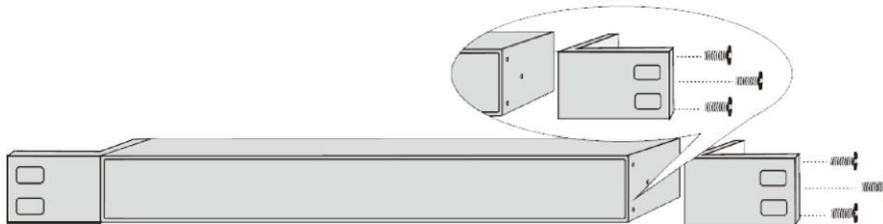
Figure 2-1 Fix L-Shaped Brackets
