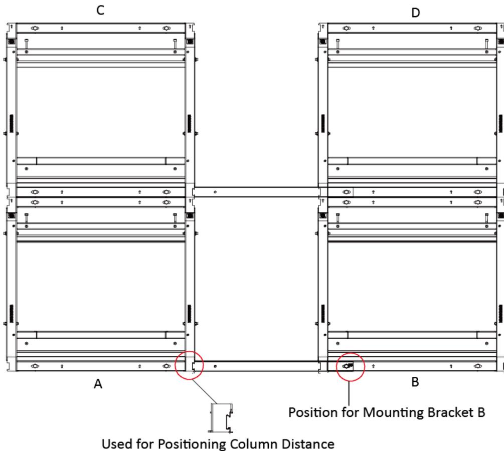
Figure 2-3 Determine Mounting Position for Bracket B
