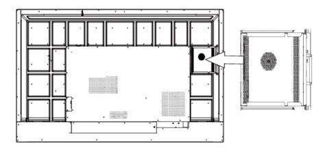
**Figure 3-7 Computer Installation**
