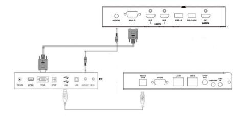
Figure 3-5 VGA Connection
