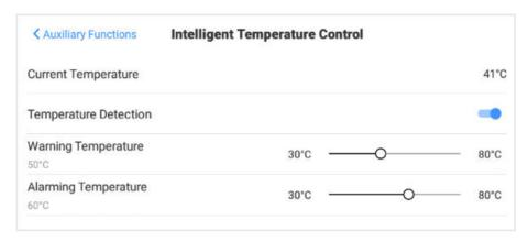
Figure 6-13 Intelligent Temperature Control
