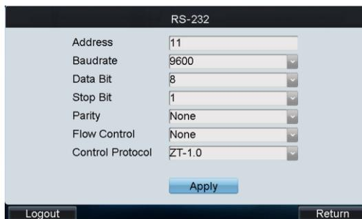
Figure 6.33 Set RS-232 Parameters
