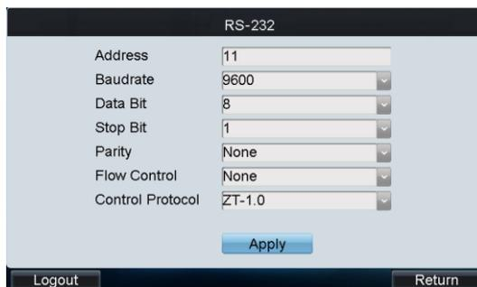
Figure 6.33 Set RS-232 Parameters
