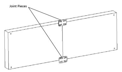
Figure 2-26 Fix the Screen with Joint Pieces
