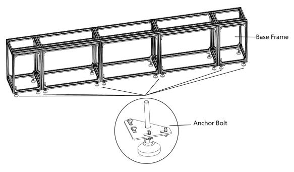
Figure 2-35 Assemble the Base Frame
