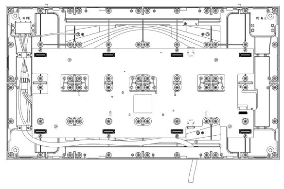
Figure 3-23 Front View of External Power Cord Connection
