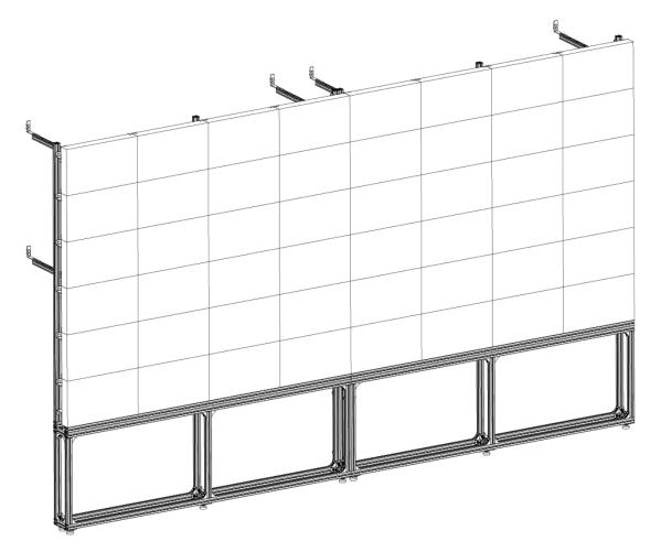
Figure 2-29 Screen Installation Finished
