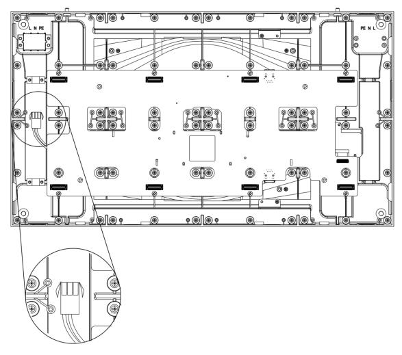
Figure 3-18 Remove the Original Power Cord
