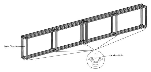
Figure 2-14 Assemble the Base Frame
