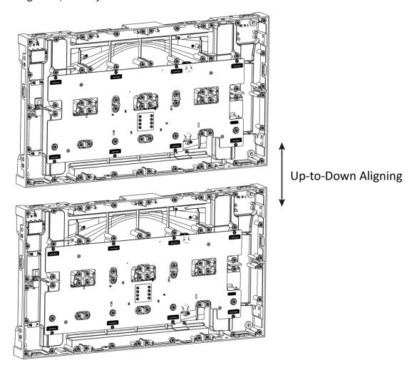
Figure 3-5 Align the Cabinet Vertically
