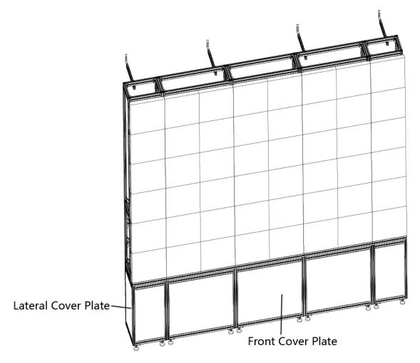
**Figure 2-52 Install the Cover Plates**
