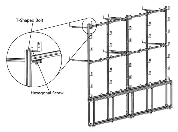
**Figure 2-25 Install the Connectors**
