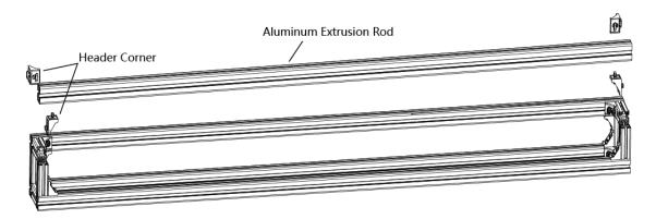
Figure 2-1 Assemble the Base Frame
