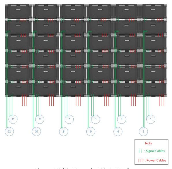
Figure 3-15 Cabling Diagram for 16 Output Interfaces
