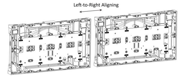
Figure 3-3 Align the Cabinet Horizontally
