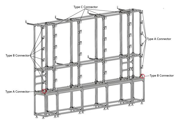
**Figure 2-46 Connectors Installed**
