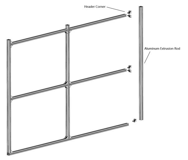
Figure 2-16 Assemble the Rack Frame Unit
