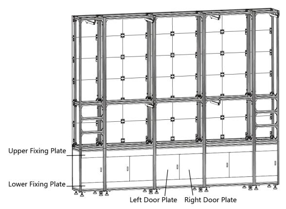
Figure 2-53 Install the Door Plates
