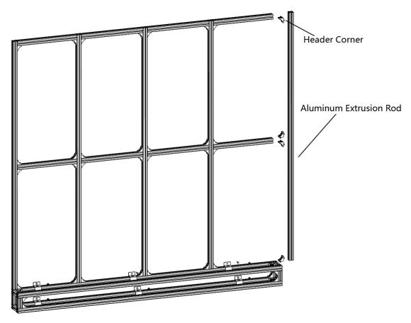
Figure 2-4 Assemble the Rack Frame
