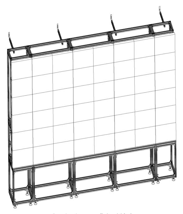
Figure 2-51 Screen Installation Finished
