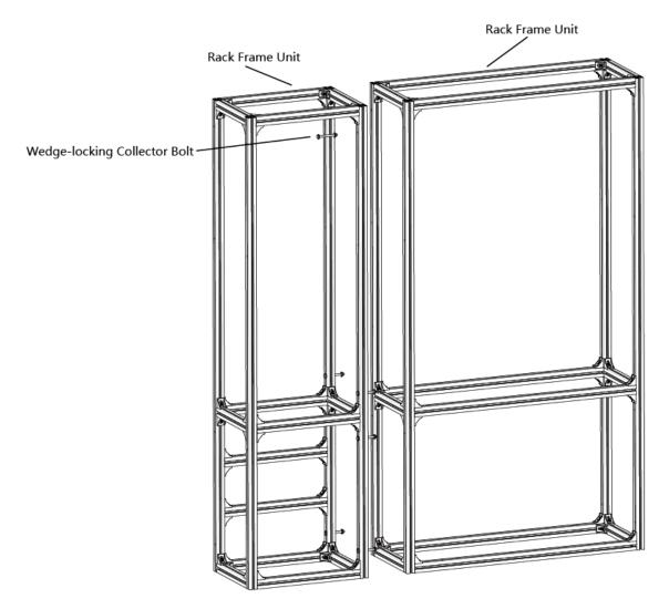
**Figure 2-38 Connect the Rack Frame Units**
