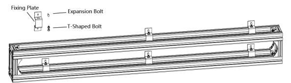
Figure 2-3 Fix the Base Frame onto the Wall
