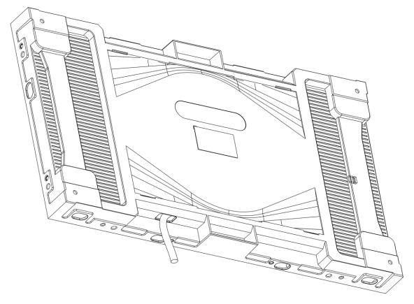
Figure 3-24 Rear View of External Power Cord Connection
