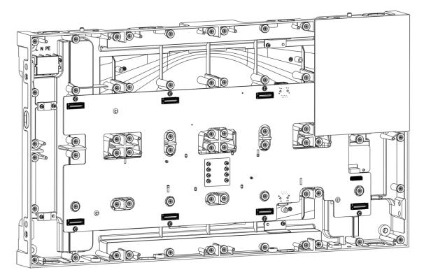
Figure 3-9 Install the First Lamp Board
