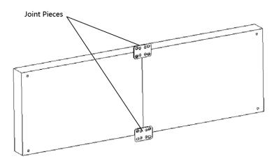
Figure 2-48 Fix the Screen with Joint Pieces
