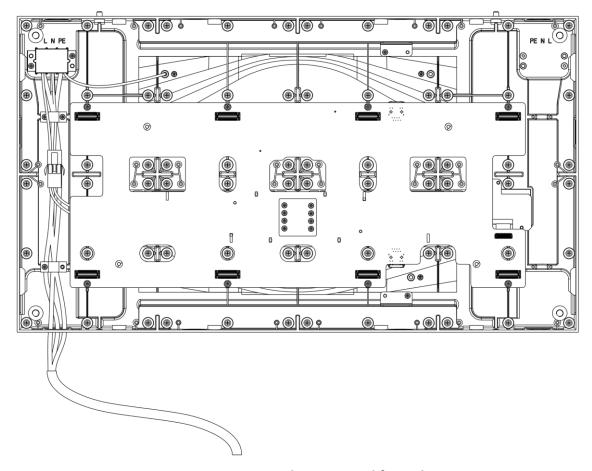
Figure 3-19 Connect External Power Cord from the Bottom
