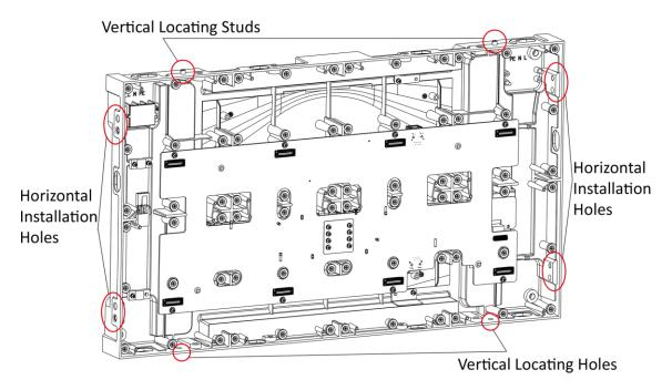
Figure 3-2 Locating Studs, Locating Holes and Installation Holes
