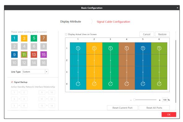
Figure 3-27 Cabling Diagram in Signal Redundancy Mode on the Client
