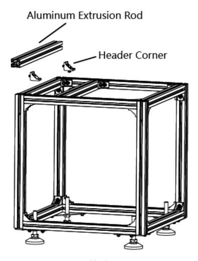
Figure 2-30 Assemble the Base Frame Unit
