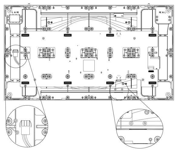
Figure 3-21 Remove the Original Power Cord and Baffle
