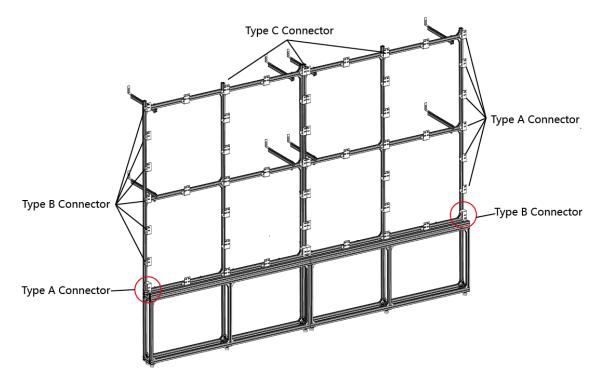
**Figure 2-24 Connectors Installed**
