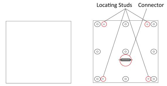
Figure 3-7 Front and Back of the Lamp Board
