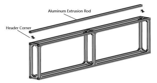
Figure 2-11 Assemble the Base Frame Unit
