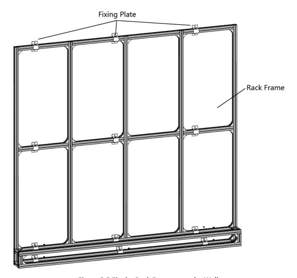
Figure 2-5 Fix the Rack Frame onto the Wall
