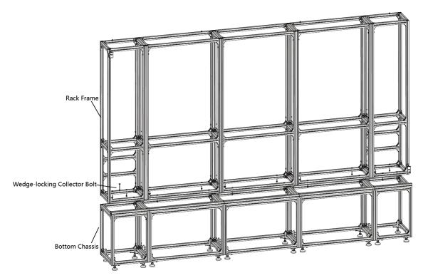
Figure 2-40 Align the Rack Frame to the Base Chassis
