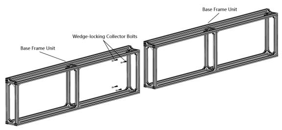
Figure 2-13 Connect the Base Frame Units
