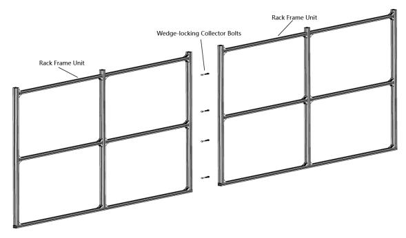
Figure 2-17 Connect the Rack Frame Units
