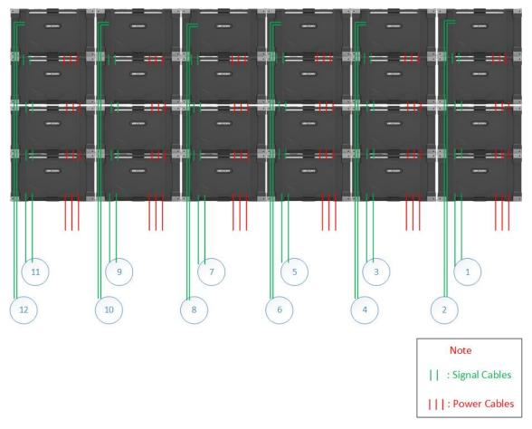
Figure 3-26 Cabling Diagram in Signal Redundancy Mode
