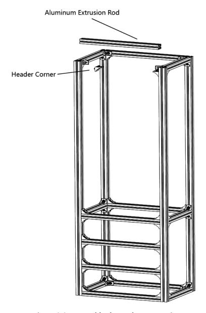
Figure 2-37 Assemble the Rack Frame Unit
