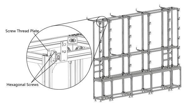
**Figure 2-47 Install the Connectors**
