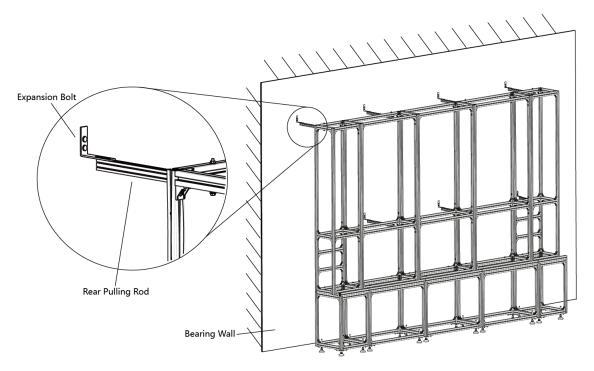
Figure 2-44 Fix the Rear Pulling Rods onto the Bearing Wall
