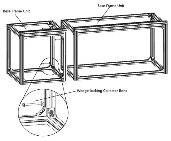
Figure 2-32 Connect the Base Frame Units
