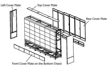
Install the left, right, front, rear, and top cover plates respectively.
