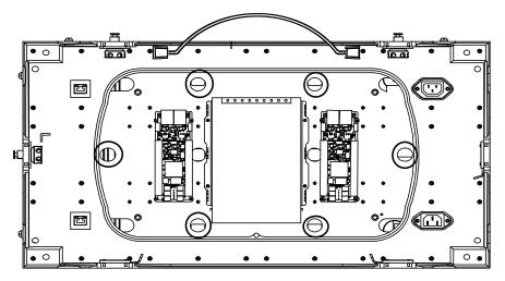
Figure 3-18 Through Holes inside the Cabinet
