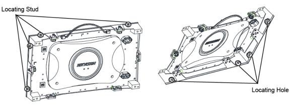
Figure 3-10 Locating Studs and Locating Holes on Cabinets
