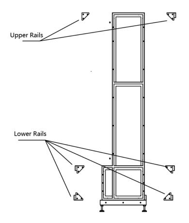
Figure 2-6 Side View of Rail Installation
