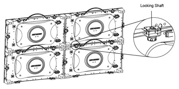
Figure 3-13 Push the Locking Shafts
