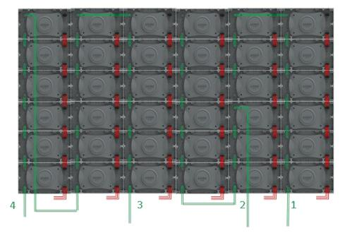
Figure 3-21 Cabling Diagram for Four Output Interfaces
