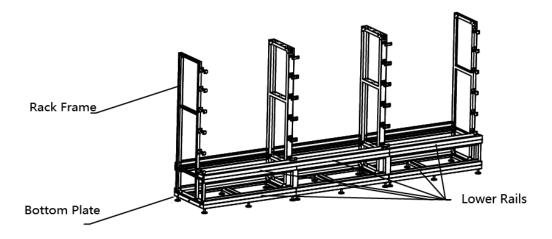
Figure 2-4 Install the Lower Rails
