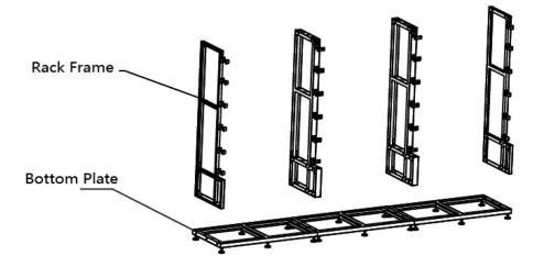
Figure 2-3 Install the Rack Frames
