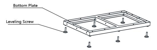
Figure 2-1 Assemble the Bottom Plates
