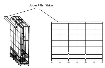
Figure 2-11 Install the Upper Filler Strips
