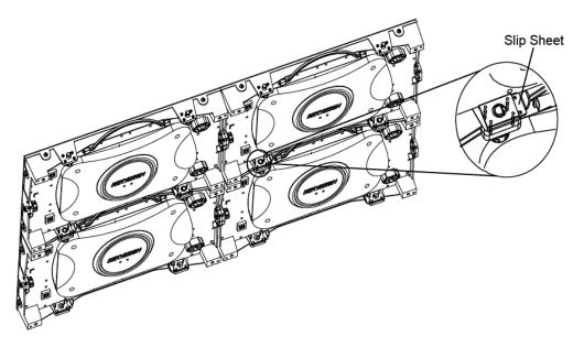
Figure 3-14 Slide the Slip Sheets
