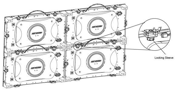
Figure 3-15 Rotate the Locking Sleeves Clockwise
