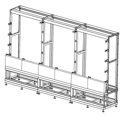
Figure 3-6 Installation of the Lowest Row Finished
