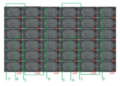
Figure 3-23 Cabling Diagram in Signal Redundancy Mode
