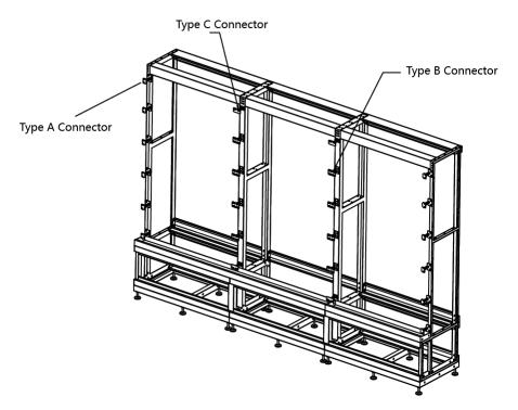
Figure 2-9 Install the Connectors
