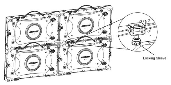
Figure 3-12 Rotate Lock Sleeves Anticlockwise
