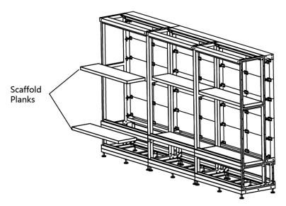
Figure 2-12 Install the Scaffold Planks
