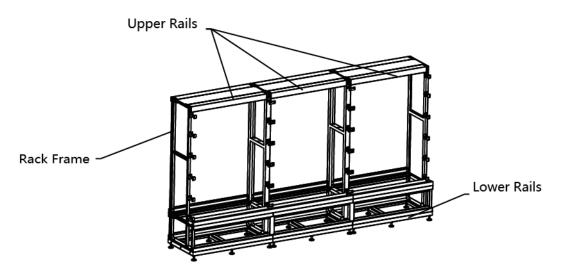
Figure 2-5 Install the Upper Rails
