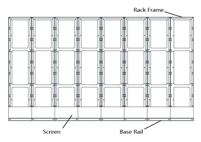
Figure 2-17 First Row of Screens Installed
