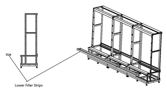
Figure 2-7 Install the Lower Filler Strips
