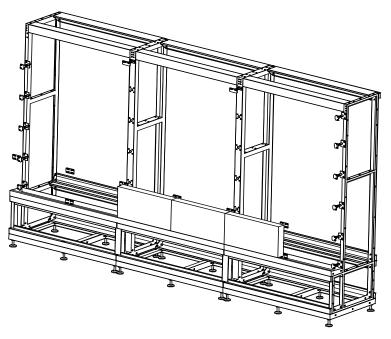
Figure 3-5 Install Screens from Middle to Sides
