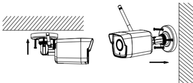
Figure 3-3 Install the Camera
