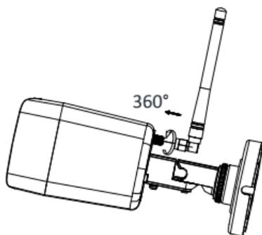
Figure 3-1 Install the Antenna
