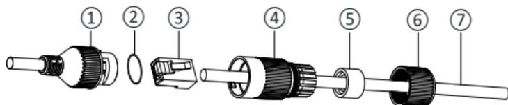
Figure 3-5 Waterproof Accessory Components
