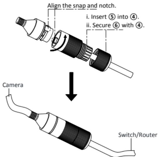
Figure 3-6 Waterproof Accessory Installation
