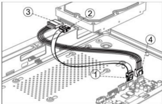
Figure 2-2 Connect Cables
