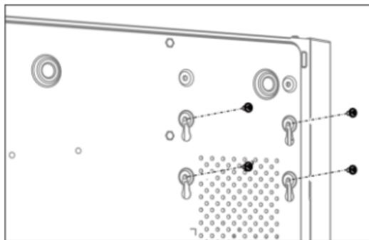
Figure 2-3 Fix HDD to Device Bottom
