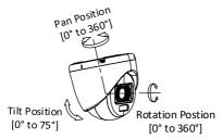
Figure 2-15 3-Axis Adjustment
