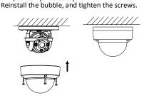
Figure 2-15 Bubble Reinstallation
