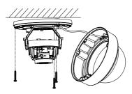
Figure 2-2 Install Mounting Base
