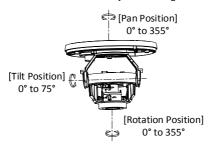
Figure 2-3 3-Axis Adjustment
