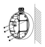
Figure 2-22 Secure Junction Box's Body
