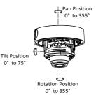
Figure 2-14 3-Axis Adjustment 8. Fit the bubble back to the camera.
