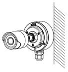
Figure 2-8 Combine the Junction Box's Cover with its Body
