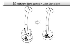
Figure 3-2 Fix Camera to Wall Mount
