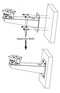
Figure 2-1 Install Wall Mounting Bracket
