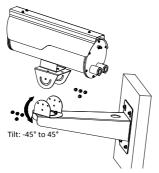
Figure 2-5 Adjust Tilting Position
