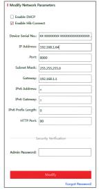
Figure 3-5 Modify the IP Address
