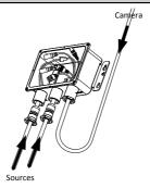
Figure 2-11 Fix Wall Mounting Bracket to Wall
