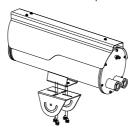
Figure 2-3 Fix the Camera to the Pedestal
