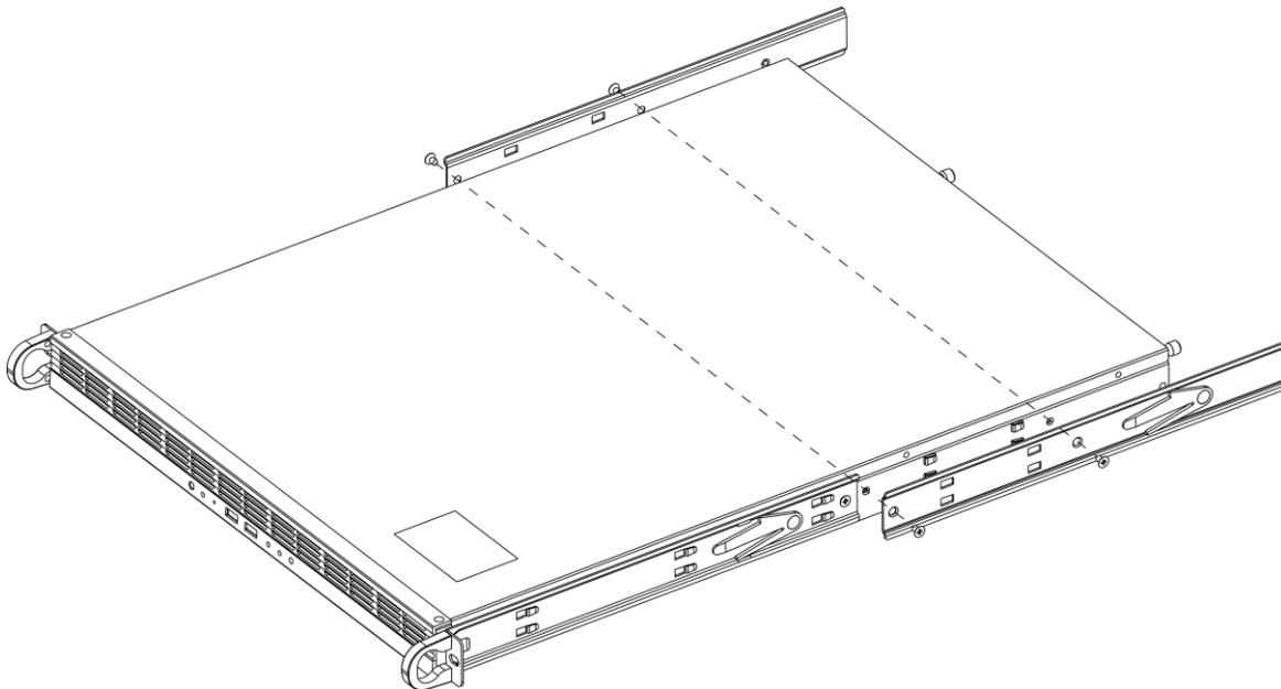
Figure 2-1 Fix Server and Inner Rails
