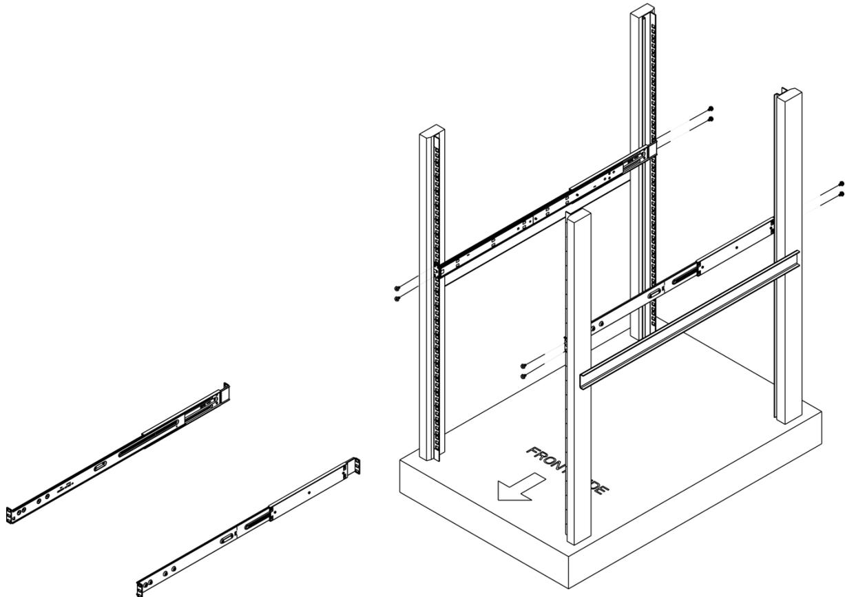
Figure 2-2 Install Outer Rails
