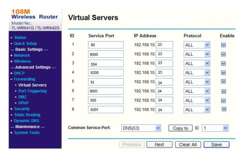
**Figure 9-1 Port Mapping on Router**
