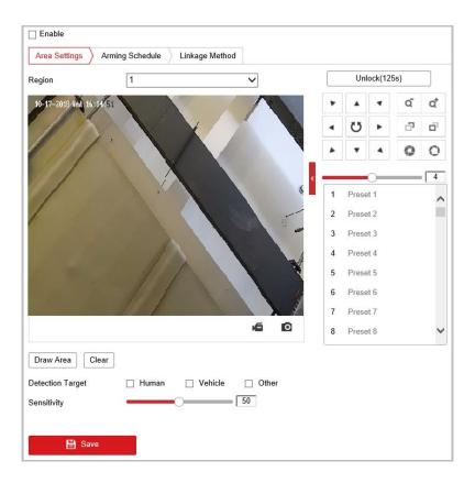
Figure 5-26 Configuring Region Exiting Detection
