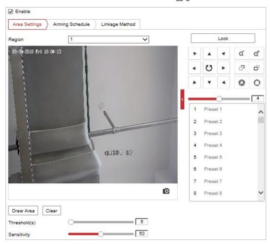
Figure 5-27 Configuring Region Exiting Detection
