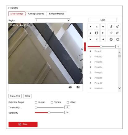
Figure 5-23 Configuring Intrusion Area
