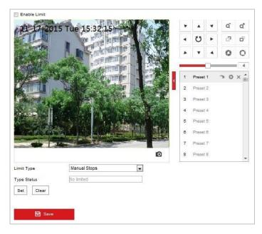
Figure 5-29 Configure the PTZ Limit
