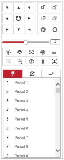
Figure 4-4 PTZ Control Panel
