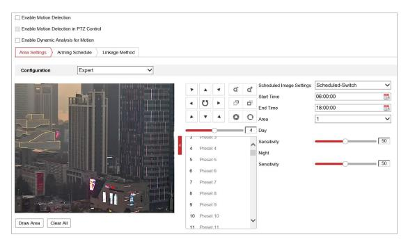
Figure 5-11 Motion Detection Settings-Expert
