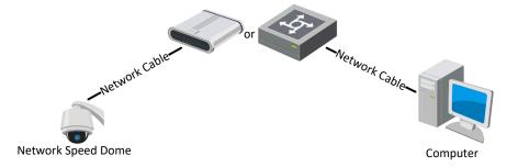
Figure 2-2 Connecting via a Switch or a Router
