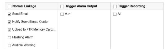
Figure 5-15 Linkage Method
