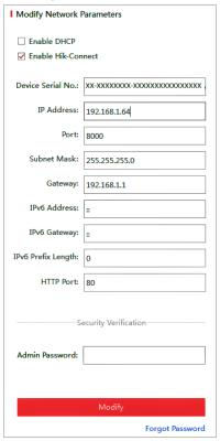
Figure 2-5 Modify the IP Address
