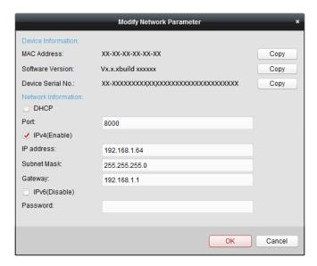
Figure 2-9 Modifying the Network Parameters
