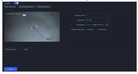
Figure 5-11 Line Crossing Detection
