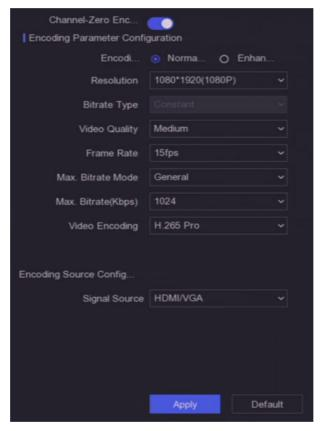
Figure 6-35 Channel-Zero Encoding
