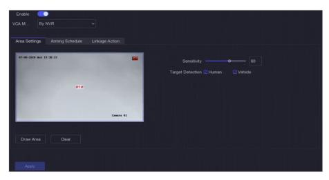
Figure 5-10 Motion Detection
