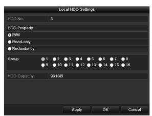
Figure 12-13 Local HDD Settings Interface
