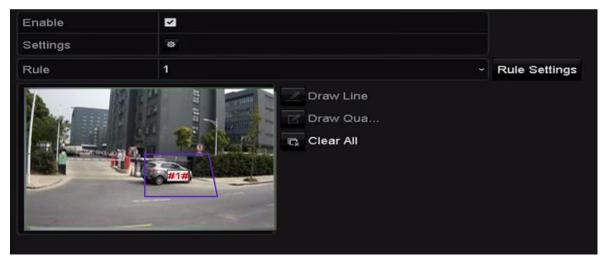
Figure 9-6 Draw Area for Intrusion Detection
