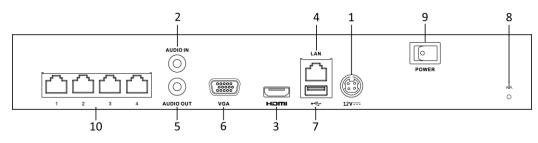
Figure 1-7 DS-7600NI-Q1/4P and DS-7604NI-K1/4P(B) Series
