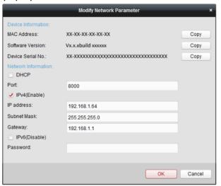
**Figure 1-6 Modify Network Parameters**
