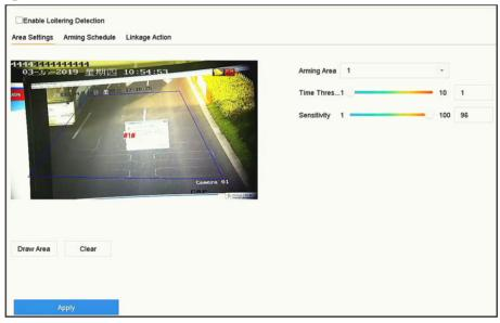
**Figure 5-7 Loitering Detection**
