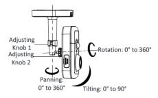
Figure 3-12 Adjust the Camera
