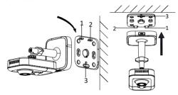
Figure 3-11 Buckle the Camera into Adapter Plate
