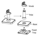
Figure 3-6 Disassemble the Bracket
