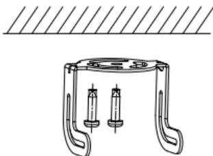
Figure 2-4 Fix the Bracket on the Ceiling
