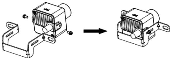
Figure 2-7 Fix the Bracket to the Camera
