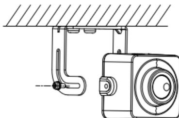
Figure 2-5 Fix the Camera to the Bracket
