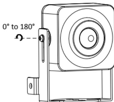
Figure 2-3 Fix the Bracket
