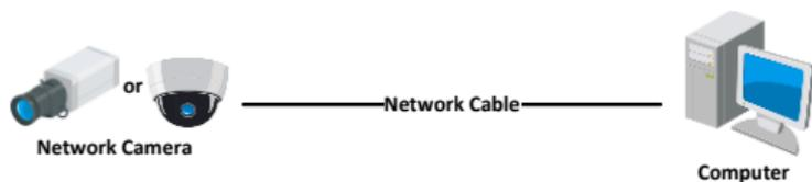
Figure 3-1 Connect Directly
