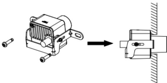
Figure 2-8 Install the Camera to the Wall
