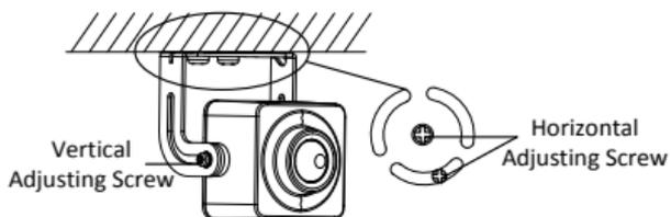
Figure 2-6 Adjust the Camera Angle
