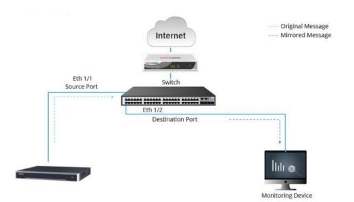
Source port should be the LAN connect to NVR/DVR or the cable connect to main Source (e.g. Video guard) Monitor Port, which connect to Laptop or PC, which run Wireshark or other capture tool .
