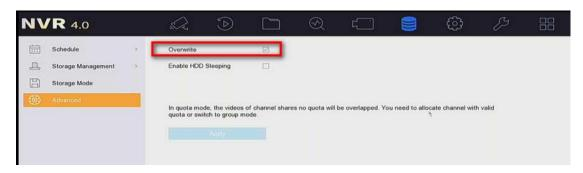
If overwrite not enabled we will receive HDD full alarm.
