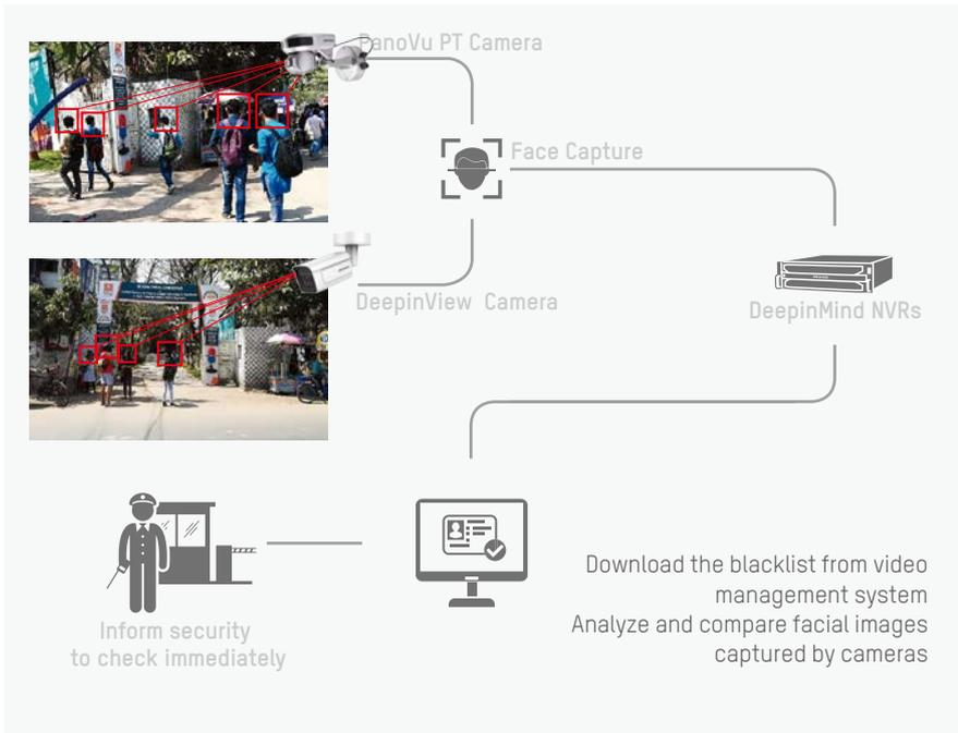
Through front-end cameras, the platform can perform real-time monitoring, face image capture, and alarm configuration.
