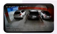
Operators can search the Parking Guidance Camera footage via the Parking Control Panel by time, to see activity in the car park, if there's an incident. So, if something happens at a particular time, an operator can see if there were any alerts at that time, and investigate.
