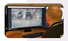
Operators can search for license plates in the HikCentral VMS using ANPR data from the Parking Guidance Camera, increasing security and providing a useful feature if an incident occurs. For example, a 'hit and run' accident could be investigated. This data is also used by a Parking Inquiry Machine (see below).
