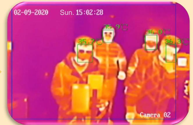
Fast temperature screening with elevated temperature alarm (pop-up image/audio warning)
