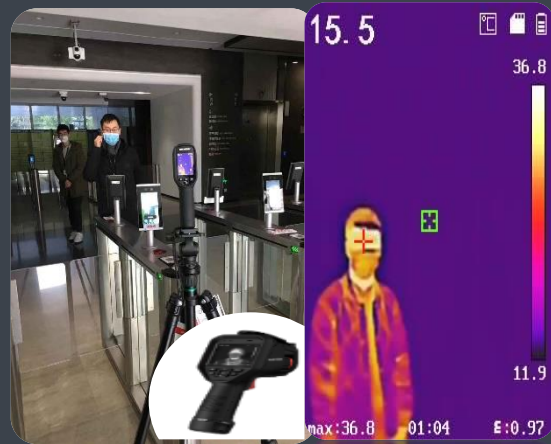
Portable infrared temperature measurement at entrances of building
