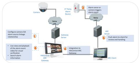
Configure the linkage relationship between 3rd party alarm source and Hik-camera source on the HikCentral Web Client, e.g., Alarm Zone F of Area A links to Camera 01.
