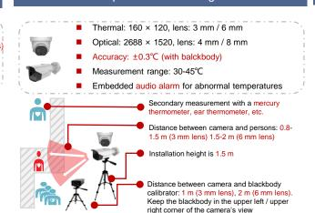
Temperature stability: ±0.1°C/h; Effective emissivity: 0.97±0.02; Operating temperature: 0-30°C
