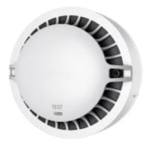
JTY-GF-HK1014 is a 4-wire smoke&heat detector, the device supports dual-light smoke detection for more accurate detection, and alarm linkage output switch signal. Fire alarm can be used to link security network video recorders, cameras, intrusion alarm panels, access controller, dynamic environment monitoring and other equipment. It is not suitable for installation in places where there will generate a lot of black smoke, large amounts of dust, water mist, steam, oil mist, smoke retention, etc.
