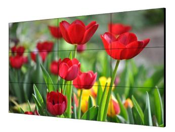
The DS-D2055UL-1B LCD display uses an industry-level ultra-narrow bezel design, which enables a bezel width of 3.5 mm between neighboring displays. The adopted direct-lit LED backlighting technology helps achieve ultra-high and uniform brightness of 500 cd/m² without boundary shadows. The display has abundant interfaces for video inputs, such as DVI, VGA, HDMI, and DP.
