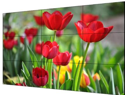
The DS-D2055UL-0A LCD display uses an industry-level extreme-narrow bezel design, which enables a bezel width of 3.5 mm between neighboring displays. The adopted direct-lit LED backlighting technology helps achieve ultra-high and uniform brightness of 500 cd/m<sup>2</sup>. The display has abundant interfaces for video inputs, such as DVI, VGA, HDMI, and DP.
