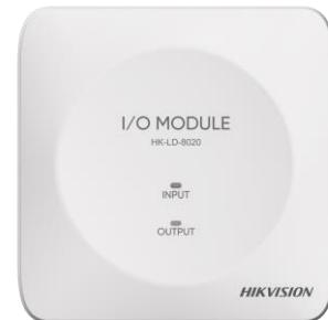
I/O Module is a very important part of the fire alarm system, which has passive contact output, normally open or normally closed input, can be used to control the electromagnetic valve, exhaust valve and other equipment, and feed the action signal of the equipment to the fire alarm control panel.
