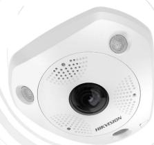
DS-2CD6365G0-IVS(D) is a fisheye network camera capable of providing a 360-degree panoramic image of its scene. The progressive scan CMOS sensor provides high-resolution images of up to  $2560 \times 2560$ . Up to 20 live view display modes, designed for 3 mount types, meet various user preferences. Three independently controlled IR lights offer a range of 15 m and provide good vision in low or even zero-light environment.
