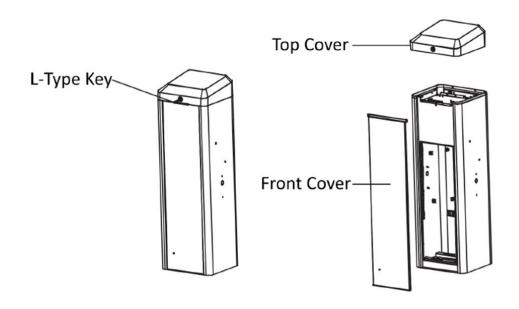
3) 通过手自动切换,分别在开到位和关到位的状态下拆掉机箱内部的两个夹头螺丝。 Through manual and automatic switching, remove the two clamp screws inside the chassis in the open and close limit respectively.
